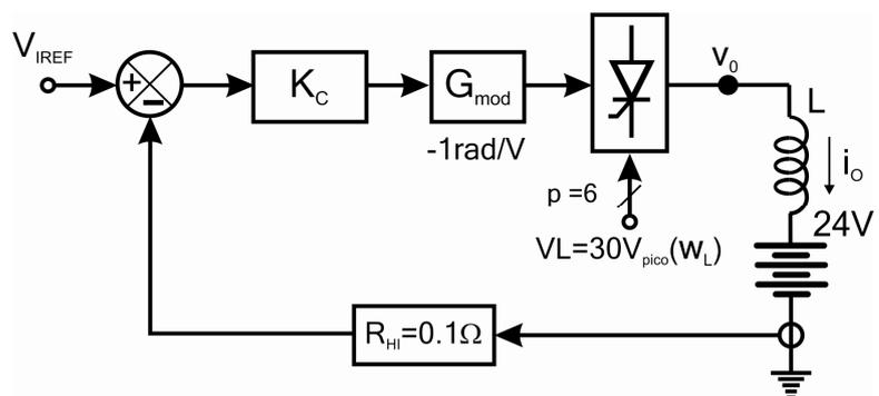
$$\frac{V_{OPP}}{V_{pico}} = 1 - \cos\left(\alpha - \frac{\pi}{p}\right) \Rightarrow 0 \leq \alpha \leq \frac{\pi}{p}$$
