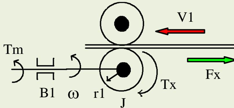
$$V_1 = \omega r_1$$
