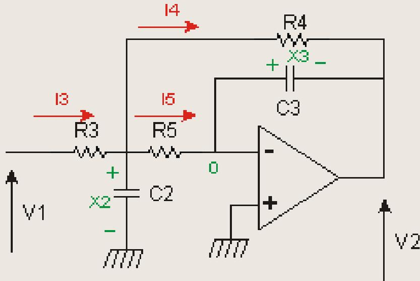
$$V_1 = I_3 R_3 + X_2 \quad ; \quad V_2 = -X_3$$
