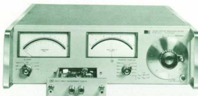
Fig. 4. Current and voltage channels and switching functions are contained in a plug-in which also contains the measurement terminals.
