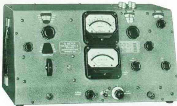
Fig. 10. Especially designed to measure Q , the -hp- Model 260A Q Meter measures Q of inductors from 10 to 625 directly over a frequency range from 50 kHz to 50 MHz.
