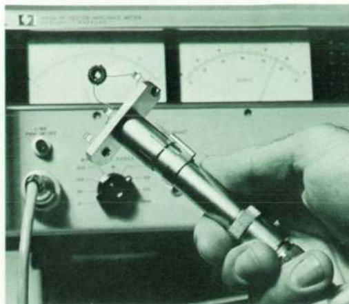
Fig. 7. Discrete components may be measured at high frequencies by clipping them to the component mounting adapter of the -hp- Model 4815A. This toroid is being checked at a frequency below resonance.
