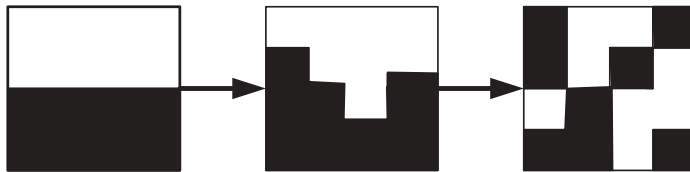
Fig. 7.1 Schematic representation of random distributive mixing (e.g., a process that takes place in a V-blender).
