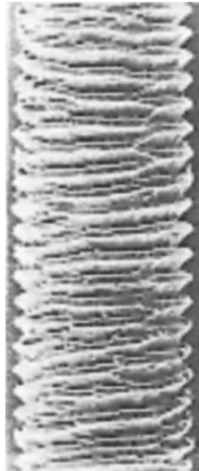
Fig. 12.17 Scanning electron micrograph of HDPE extruded at a shear rate slightly lower than the oscillation region, showing "sharkskin." [Reprinted by permission from N. Bergem, "Visualization Studies of Polymer Melt Flow Anomalies in Extruders," Proceedings of the Seventh International Congress on Rheology , Gothenberg, Sweden, 1976, p. 50.]
