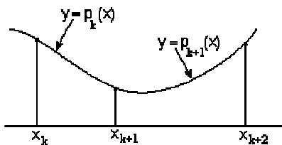
$$\text{Por (6)} \quad h_k c_k + 2(h_k + h_{k+1})c_{k+1} + h_{k+1}c_{k+2} = \frac{3}{h_{k+1}}(a_{k+2} - a_{k-1}) - \frac{3}{h_k}(a_{k+1} - a_k)$$
